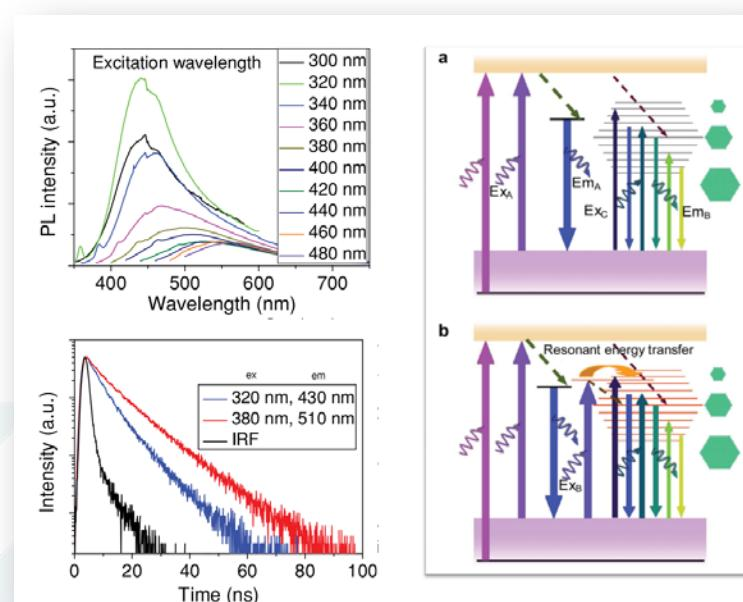
**Schematic illustration of the PL emission mechanism**
