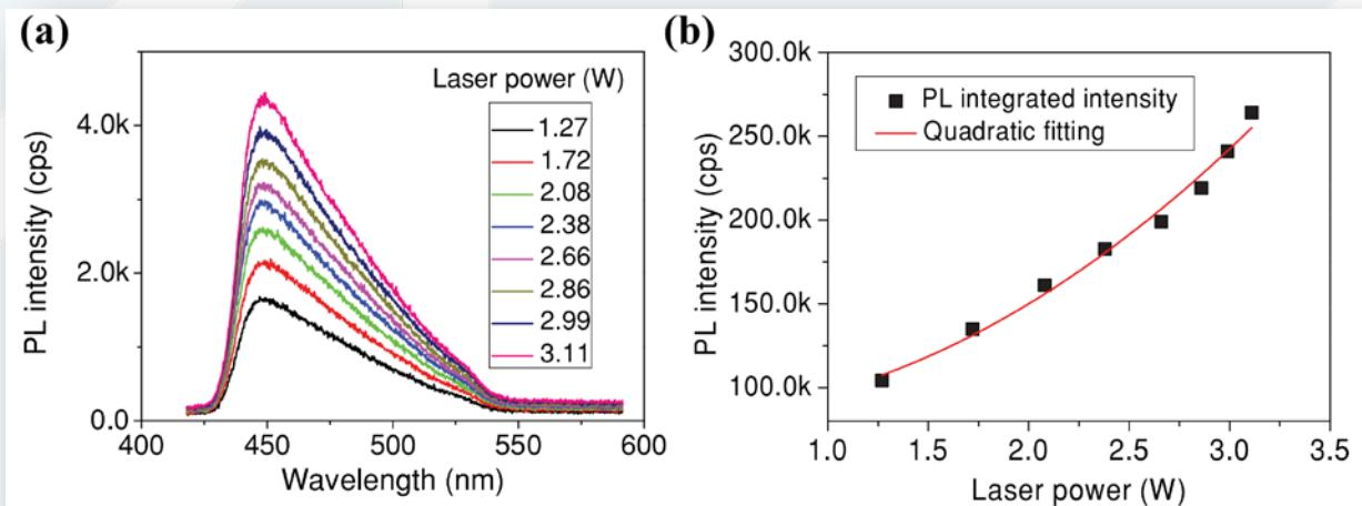
(a) UCPL spectra obtained from GQDs under excitation of a femtosecond pulsed laser at 800 nm. (b) UCPL integrated intensity as a function of laser power
