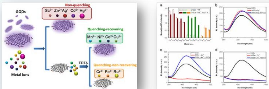
Quenching and recovering effect of transition metal ions on the photoluminescence of GQDs.
