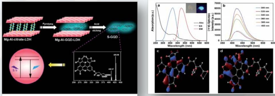
Schematic illustration of the formation of S-GQDs in the confined space of LDH
